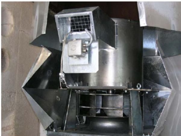
HT-SVK 630-4 before fire test from 11.07.2006; open casing
