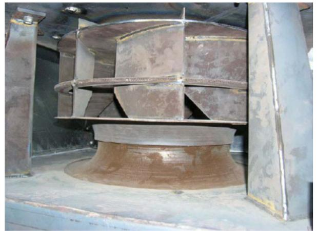
HT-SVK 630-4 after fire test from 11.07.2006; impeller
